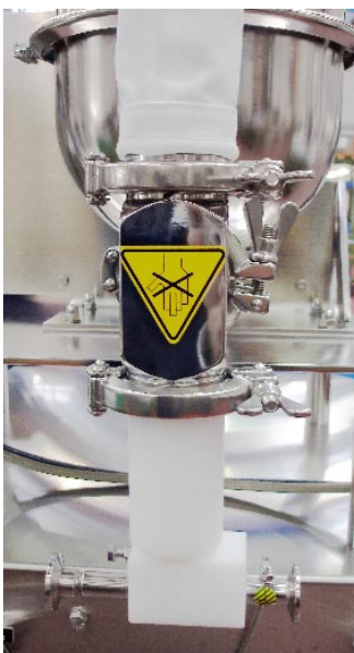
Feeder outlet with venturi injector
