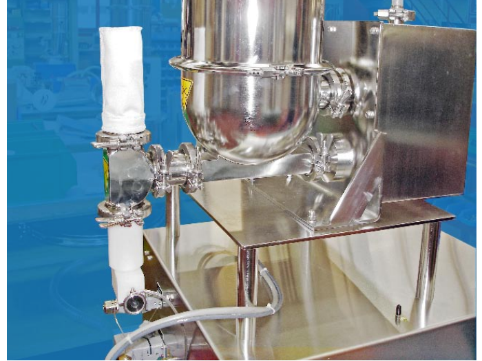
Volumetric pharmaceutical feeder with gas venturi on outlet
