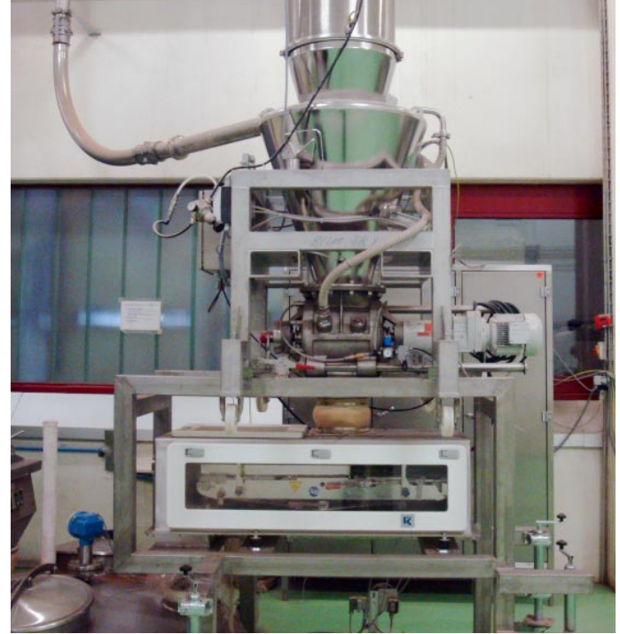
Smart Weigh Belt feeder shown with vacuum receiver, buffer hopper and AeroLock rotary pre-feeder.
